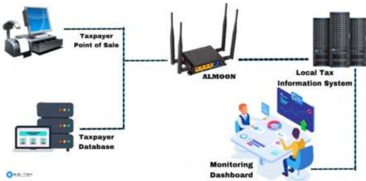
Figure 3. TMD with connection configuration to database/transaction file Source: BPPKAD of Surakarta
