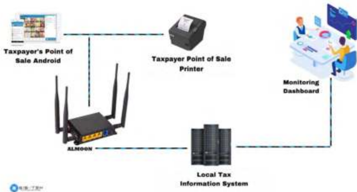
Figure 2. TMD with connection configuration to the printer of point of sales/cash register Source: BPPKAD of Surakarta
