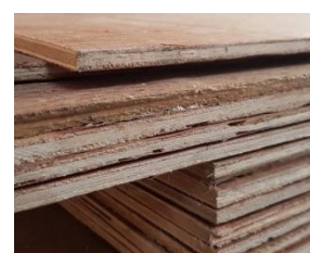
Figure 3. Defects of Plywood Thickness
