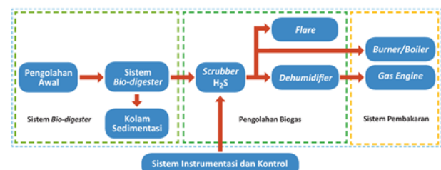
Figure 4: Processing of POME into Biogas
